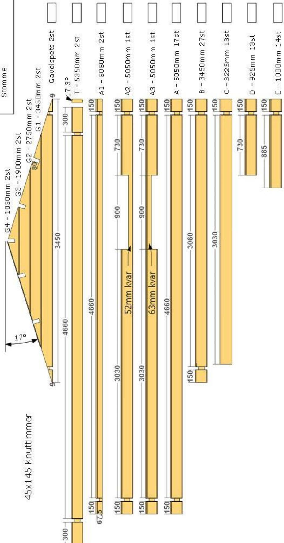
The drawing shows a gabled roof with a 17° pitch. Key dimensions include a total length of 4660mm, a peak height of 3030mm, and a base width of 3450mm. Components are labeled G1 through G4, T, A, B, C, D, and E. A 17.3° angle is also indicated at the peak.
